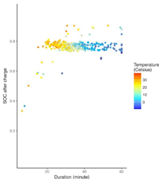
**Figure 13. Dependence of DCFC final SoC on temperature.**
