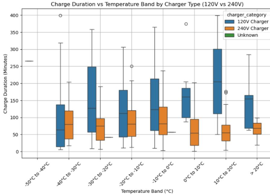
Figure B-1. Charge duration versus temperature by charger type
