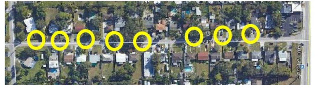
Solar lights placement study for use consulting community members prior to installation. Picture from Google Maps, modified by PUMPS [Bloetscher 2023]
