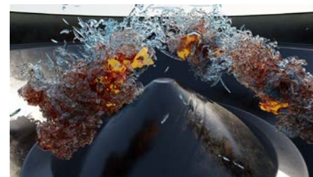
Compression ignition in a high-pressure combustion chamber, computed on Frontier as part of Exascale Computing Program Challenge Problem, 20223
