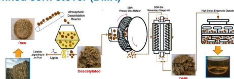
Fig. 2. Different corn stover substrates obtained from NREL pilot plant DMR pre-treatment process. Modified from Chen, X., et al. (2016).
