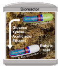
Fig. 1. Proposed process configuration for this technology. Co-cultures at 350 mL working volume are inoculated with Ctc and Ctb. Ctc will carry out the primary biomass deconstruction while Ctb will utilize solubilized sugars (including those not used by Ctc) and by-products to produce butyric acid. Cultivations were performed under anaerobic conditions, at pH 7, and 55°C.
