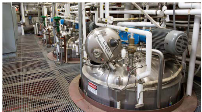
Top Photo: The IBRF pretreatment reactors (upper) and high-solids enzymatic hydrolysis reactors (lower). Photo by Dennis Schroeder, NREL 33952
