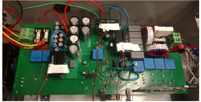
Fig. 9. Experimental setup of homegrown inverter with thermocouples
