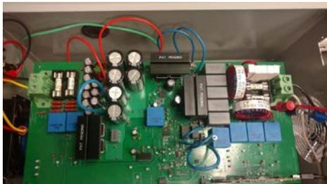
Fig. 2. Board Layout of the home-grown inverter
