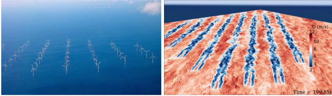
Figure 7: (a) Aerial view of the Lillgrund wind farm, and (b) simulation results showing velocity magnitude. Results were calculated with the SOWFA tool. [18]
