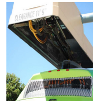
BEB docked at 500-kW overhead fast charger at Pomona Transit Center. Photo by Leslie Eudy, NREL 36044
