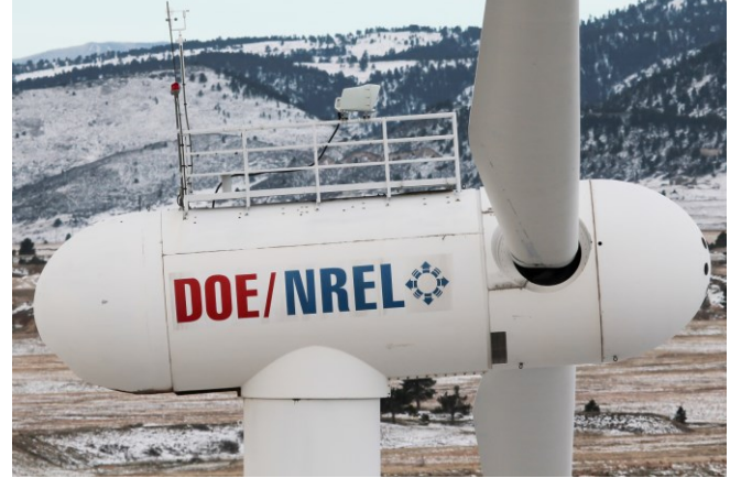
Figure 2. Avent five-beam LIDAR system mounted on the CART2. (Photo Credit: Lee Jay Fingersh, NREL 33621.)
