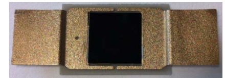
SunPower back-contact Si cell (26% @ 200x)
