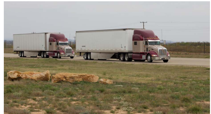
2011 Peterbilt tractors with 53-ft van body trailers (Photo courtesy of Peloton, NREL 31236)
