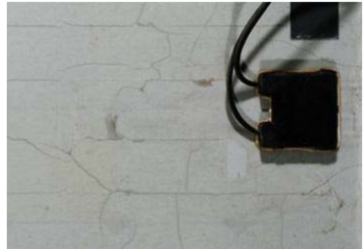
Degraded Backsheet from Gambogi SPI 2013
