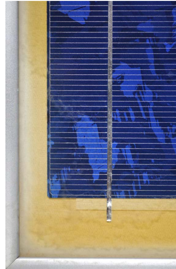
Degraded Backsheet from Gambogi SPI 2013
