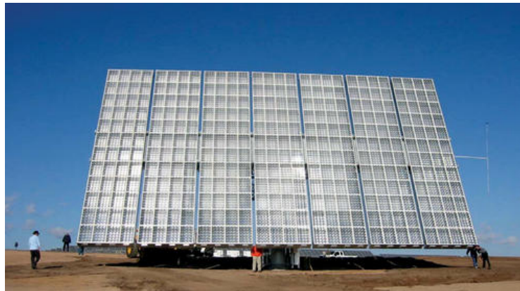
Figure A-7 Amonix: Flat Acrylic Lens Concentrator with Silicon Cells (Source: NREL)
