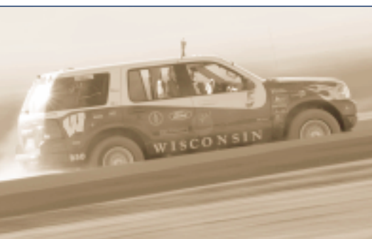
Wisconsin’s winning entry featured biodiesel hybrid-electric technology, with 45 percent better fuel economy than a stock Ford Explorer.
