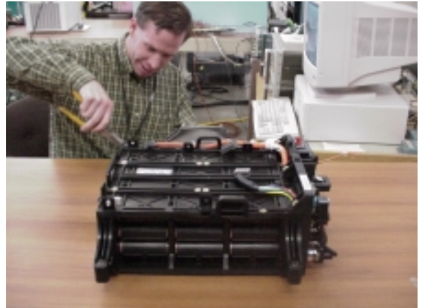
Figure 2 Insight Battery Pack Removed
