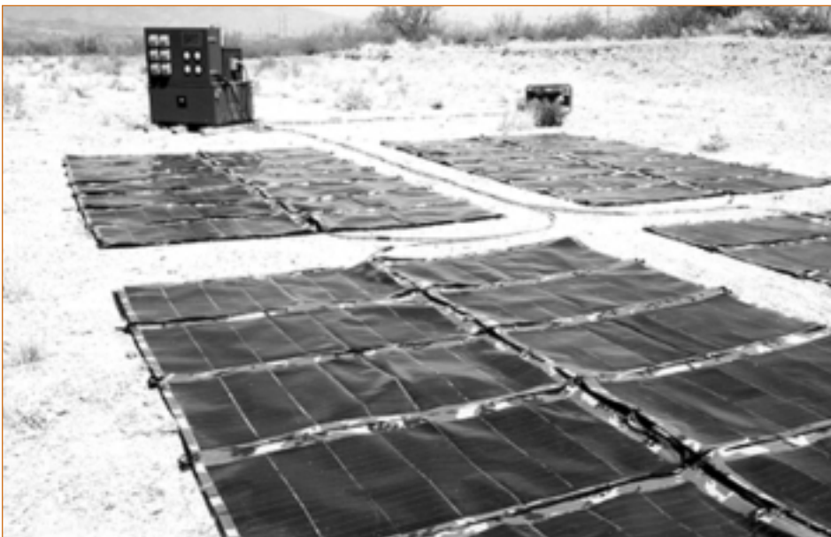
This 2.8-kW flexible solar array made of CIGS thin-film material was used in the U.S. Army's Operation Strong Angel training exercise in Hawaii. In FY 2000, Global Solar and Siemens Solar sold the first commercial products made from CIS-based thin-film materials.
