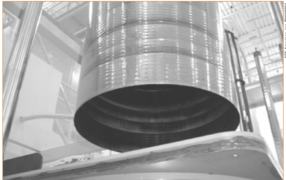
This year, the ASE Americas EFG system produced larger, 50-cm-diameter, 1.2-meter-long cylinders with walls of crystalline silicon as thin as 100 microns. Growing larger cylinders with thin walls reduces material waste and increases the speed of silicon production.
